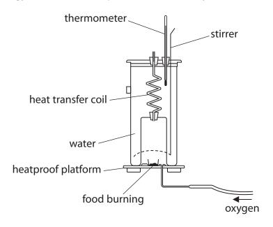
Discuss the features of this calorimeter that will give a more accurate measurement of the energy in a sample of food than the method used by the student.
