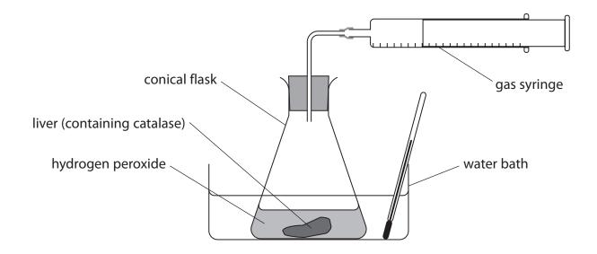
(a) (i) Describe how this apparatus can be used to investigate the effect of temperature on the activity of catalase.
