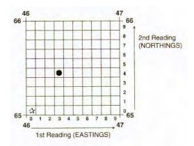
To give the six figure grid reference, first of all identify the grid square, in this case 4665. The third figure is obtained by dividing the space between grid lines 46 and 47 into ten equal parts. Similarly the sixth figure is obtained by a similar division of the gap between northings 65 and 66. This would result in a grid reference of 463654 for the dot and 460650 for the star. It should be noted that the first tenth is 0 and the last tenth is 9 in the divided grid square.
