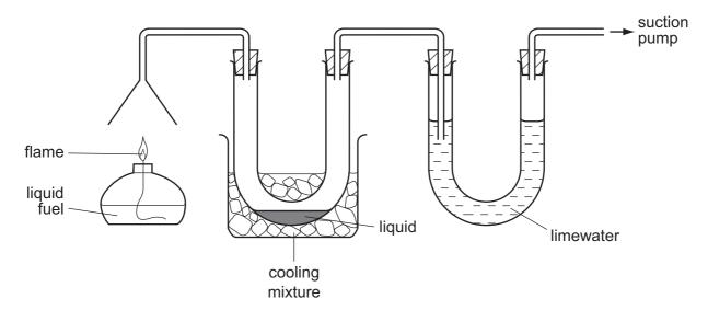
Which substances is the apparatus testing for?
