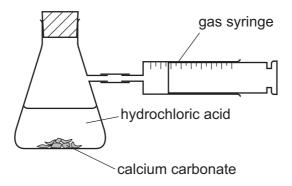
The time to collect 50 cm<sup>3</sup> of gas is measured. Using concentrated acid and lumps of calcium carbonate, the time is 150 s.
