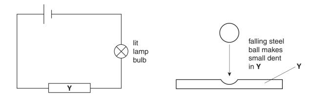
The tests show that  $\boldsymbol{Y}$  conducts electricity and is hard.
