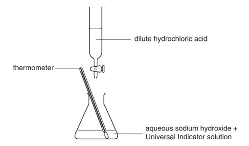
Dilute hydrochloric acid is run from a burette into the flask until a neutral solution is formed.
