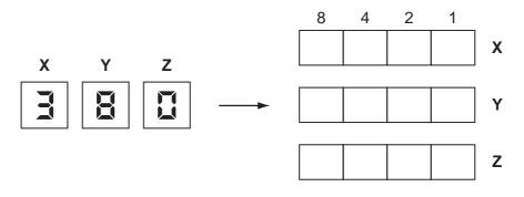
(c) If any of the 4-bit binary registers X, Y or Z contain the value 1 1 1 1 this indicates an error.
