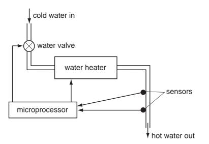
(a) Describe how the sensors and microprocessor are used to ensure the correct water flow and water temperature are maintained.
