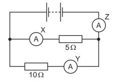
The ammeter readings are 1A, 2A and 3A.
