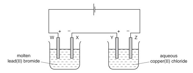
At which two electrodes would a Group VII element be formed?
