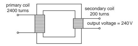
Assuming the transformer is 100 % efficient, what input voltage is needed to give an output voltage of 240 V?
