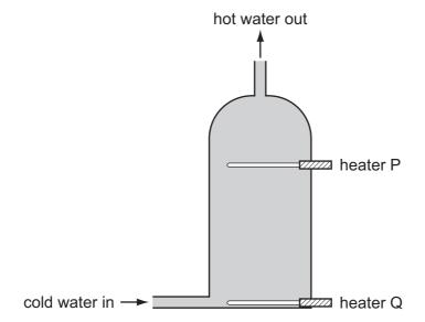
When only heater Q is switched on, it takes a very long time to heat the tank of water to the required temperature of 60 °C.
