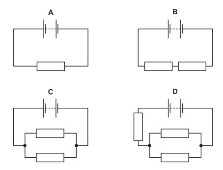
39 In the circuit below, one of the lamps breaks, causing all the other lamps to go out.
