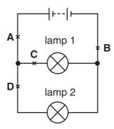
At which labelled point should a switch be placed so that lamp 1 remains on all the time and lamp 2 can be switched on and off?
