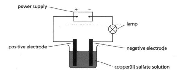
Copper forms at the negative electrode and oxygen forms at the positive electrode.
