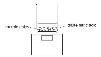
50 cm<sup>3</sup> of dilute nitric acid, an excess, was poured into a beaker. The beaker was placed on a balance and the marble chips added to the beaker. The apparatus was weighed immediately and a timer started. The mass of the beaker and contents was measured every minute for ten minutes.
