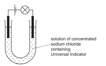
The bulb lit up. The solution near the negative electrode changed colour from green to purple.
