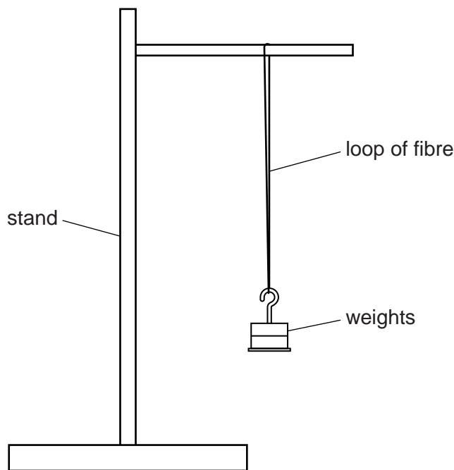
A 20 cm loop of fibre is stretched by adding weights one at a time.
