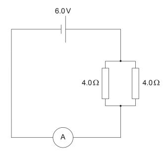
The resistance of the ammeter is  $1.0\,\Omega$ . What is the reading of the ammeter?
