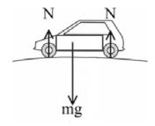
weight/gravitational force/mg/w/ $F_w/F_g$  and reaction/normal reaction/perpendicular contact force/N/R/ $F_N/F_R$  both labelled; (*do not allow "gravity" for "weight"*.) weight between wheels (in box) from centre of mass and reactions at both wheels / single reaction acting along same line of action as the weight; [2]
