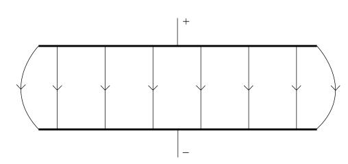
uniform (by eye) line spacing and edge effect, field lines touching both plates; downward arrows (minimum of one and none upward); [2]
