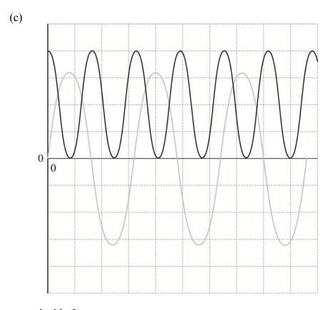
double frequency; always positive and constant amplitude; correct phase *ie* cosine squared; *A minimum of one complete, original oscillation needed to award* [3].
