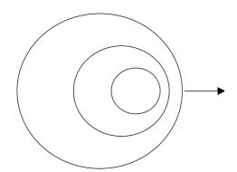
diagram showing (non concentric) wavefronts closer together in front/further apart behind source;
