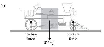
The shaded box shows the acceptable range of position for W/mg.
