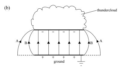
lines connecting plate and ground equally spaced in the central region of thundercloud and touching both plates; (judge by eye) edge effects shown; (accept either edge effect A or B shown on diagram)
