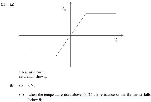
and so the voltage at the non-inverting input of the op-amp is negative; (the output voltage then saturates at -12 V) giving the required potential difference for the buzzer to sound;
