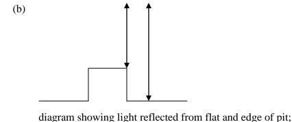
diagram showing light reflected from flat and edge of pit;if there is just the right depth;light reflected from the edge of a pit and flat interfere destructively such that thereis 0 intensity at the detector;light reflected from the flat/pits is a 0;Accept answers in terms of non-reflective pit (=0) and reflective flat/land (=1) system.
