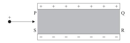
The top plate is positively charged and the bottom plate is negatively charged. There is a magnetic field in the shaded region PQRS. The particle continues to move in a horizontal straight line between the plates. Which of the following correctly describes the magnetic field direction?
