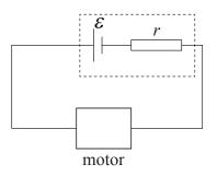
450 C of charge flows through the motor and 9000 J of energy are converted in the motor. 1800 J are dissipated in the cell. The emf of the cell is
