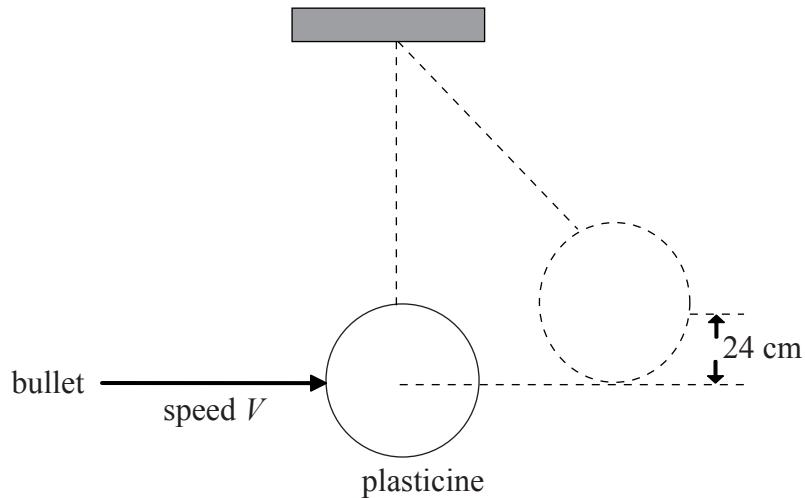
The speed of the bullet on impact with the plasticine is  $V$ . As a result of the impact, the bullet embeds itself in the plasticine and the plasticine is displaced vertically through a height of 24 cm. The mass of the bullet is  $5.2 \times 10^{-3}$  kg and the mass of the plasticine is 0.38 kg.
