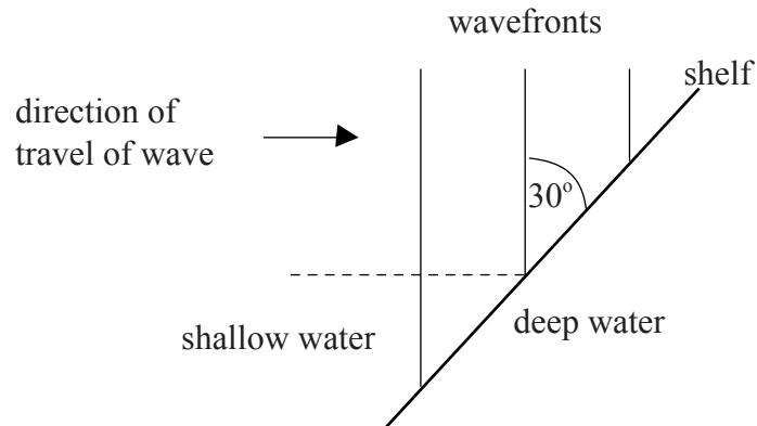
The angle between the wavefronts in the shallow water and the shelf is  $30^\circ$ . The speed of the wave in the shallow water is  $15 \text{ cm s}^{-1}$  and in the deeper water is  $20 \text{ cm s}^{-1}$ . For the wave in the deeper water, determine the angle between the normal to the wavefronts and the shelf.
