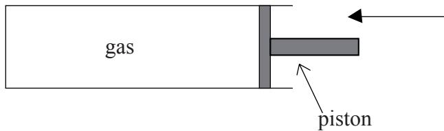
The piston is moved rapidly in the direction shown such that it compresses the gas. As a result, the temperature of the gas increases.
