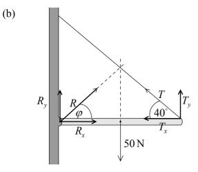
resolve horizontally:  $T_x = 39 \cos 40^\circ = 30 \text{ N}$  $|R_x| = |T_x| = 30 \text{ N}$ ;
