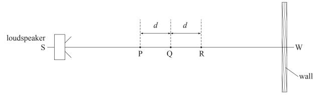
When a microphone is moved along the line SW, minimum loudness of sound is detected at points P, Q and R. There are no other minima between these points. The separation of the minima is *d*.
