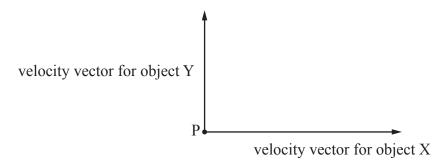
Which of the following velocity vectors best represents the velocity of object X relative to object Y?
