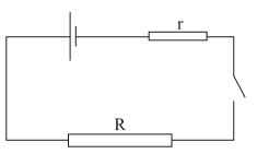
The energy transfer in the internal resistance r of the battery is 15 J when a charge of 40 C passes through it. For the same amount of charge, 45 J of energy is transferred in the resistor R.
