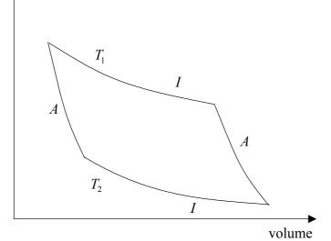
correct labelling of the axes; two sensible isotherms; two sensible adiabatics; [3 max] Use judgement for drawing of cycle. Award [2] for a good diagram, [1] for a reasonable diagram and [0] for a poor diagram.
