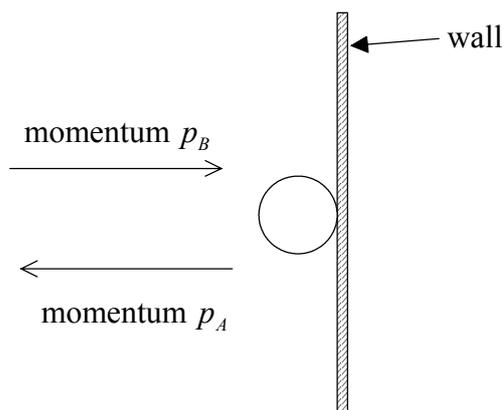
The magnitude of the momentum of the sphere just before impact is  $p_B$  and just after impact is  $p_A$ . The sphere is in contact with the wall for time  $t$ . The magnitude of the average force exerted by the wall on the sphere is
