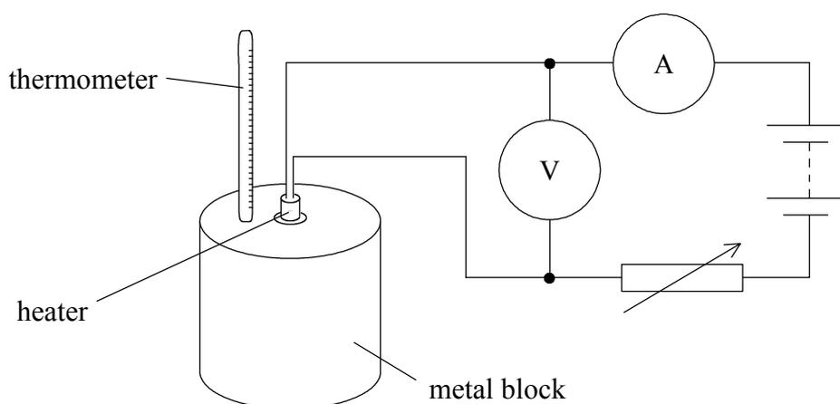
The specific heat capacity of a metal block of mass  $m$  is determined by placing a heating coil in its centre, as shown in the diagram above.
