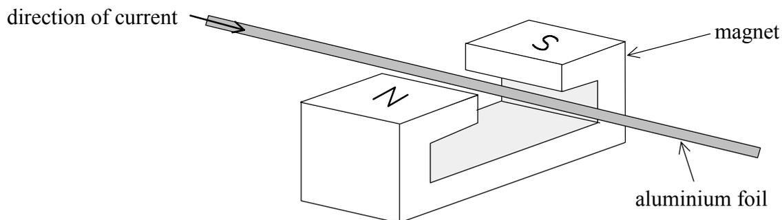
When a current is passed through the aluminium foil in the direction shown, the foil is deflected. In which direction is this deflection?
