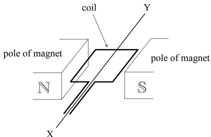
A current is passed through the coil by means of a commutator connected to the ends of the coil. What is the position of the coil in the magnetic field so that its turning effect is a maximum and what is the position of the coil when the current is reversed so that the coil rotates continuously?
