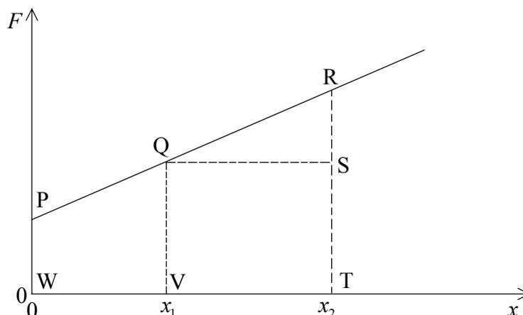
Which area represents the work done by the force when the displacement changes from  $x_1$  to  $x_2$ ?
