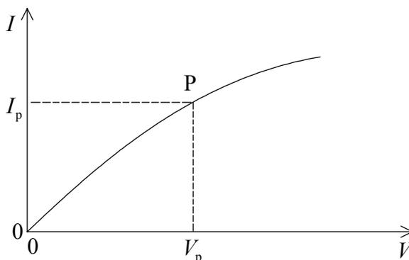
At point P, the current is  $I_p$ , the potential difference is  $V_p$  and the gradient of the tangent to the curve is  $G$ . What is the resistance of the lamp at point P?
