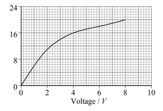
The resistance of the filament at 4.0 V is
