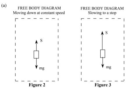
Force S is exerted by the scale, force mg is exerted by the Earth;
