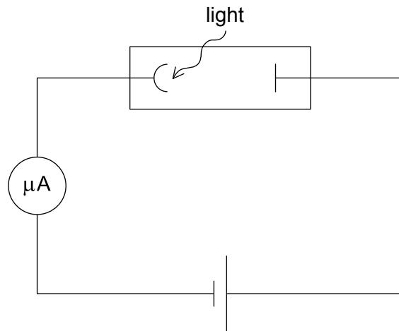
Radiation with a greater photon energy than that in (b) is now incident on the photocell. The intensity of this radiation is the same as that in (b).
