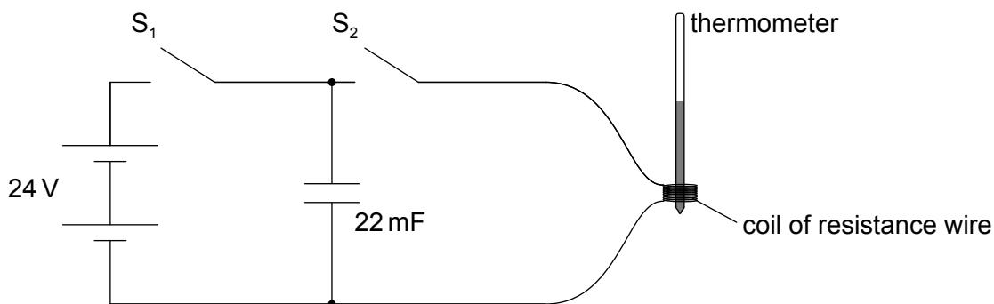
A power supply of emf (electromotive force) 24 V and of negligible internal resistance is connected to a capacitor and to a coil of resistance wire using an arrangement of two switches. Switch  $S_1$  is closed and, a few seconds later, opened. Then switch  $S_2$  is closed.
