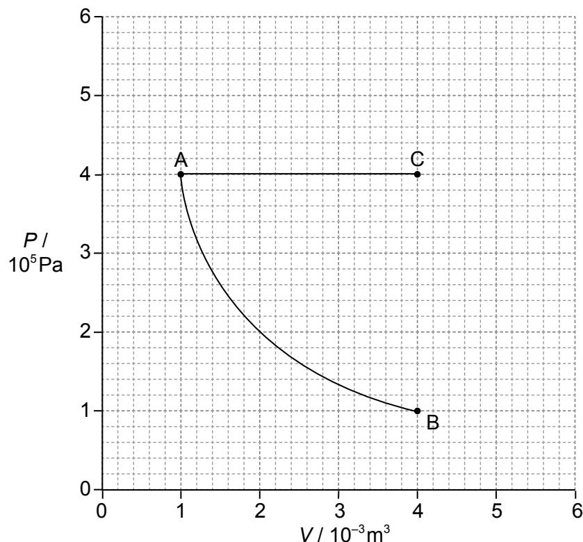
The temperature at A is 350 K. An identical mass of the same ideal monatomic gas undergoes an isobaric change from A to C.
