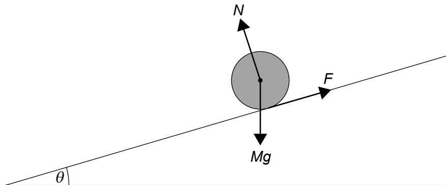
The diagram shows the three forces acting on the cylinder.  $N$  is the normal reaction force and  $F$  is the frictional force between the cylinder and the slope.
