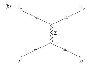
arrows for  $e^-$  point forward in time and arrows for  $\overline{\nu}_{\mu}$  point backwards in time;
