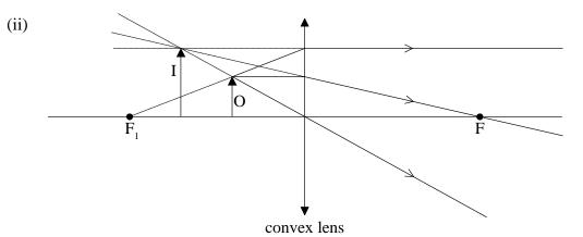
any correct ray of the three shown in the diagram;<br/>second ray correct;<br/>image shown correctly, between O and F1;[3]Accept rays without arrows and solid construction lines back to the image.
