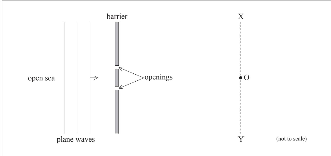
Plane water waves from the open sea are incident on the barrier and the openings act as point sources of waves. The distance from the openings to XOY is much greater than the wavelength of the wave. O is equidistant from the openings.
