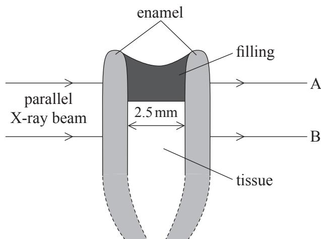
$$\text{Attenuation coefficient of filling} = 6.3 \text{ mm}^{-1}$$
