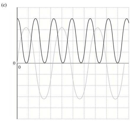
double frequency; always positive and constant amplitude; correct phase *ie* cosine squared;
