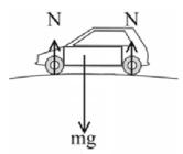
weight/gravitational force/mg/w/ $F_w/F_g$  and reaction/normal reaction/perpendicular contact force/N/R/ $F_N/F_R$  both labelled; *(do not allow "gravity" for "weight".)* weight between wheels (in box) from centre of mass and reactions at both wheels / single reaction acting along same line of action as the weight;
