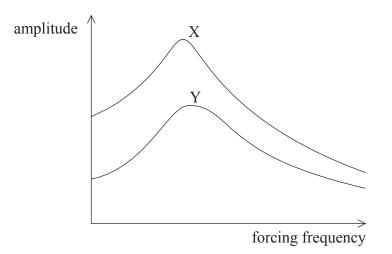
Which of the following correctly identifies the system that has the greater amount of damping and the greater natural frequency of oscillation?
