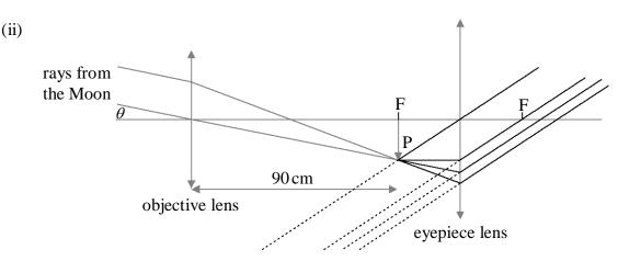
first construction line or ray; (*judge by eye*) second construction line or ray; extension of these to the left as parallel lines;
