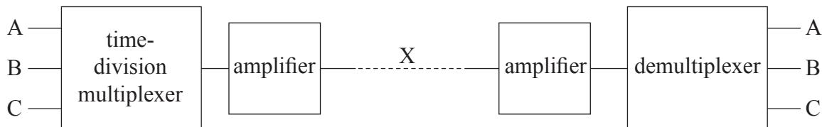
Explain how large numbers of sampled digital audio signals can be sent along the single optic fibre X.
