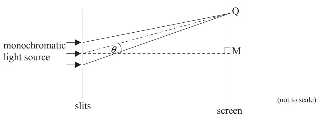
The separation of the slits is large compared to their width. A pattern of light and dark fringes is observed on the screen.
