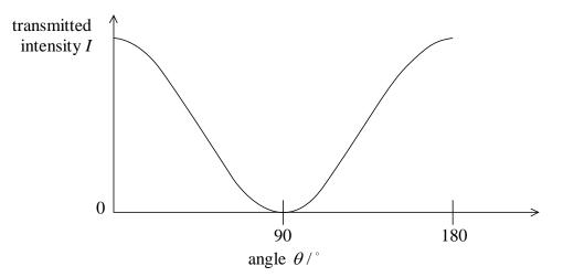
(b) solution placed between two crossed polarizer; plane of polarization rotated by an amount that depends on concentration; rotation of second polarizer/intensity of transmitted light is a measure of concentration;
