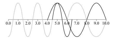
maximum displacement where two crests meet, *i.e.* at 5.0 m;
