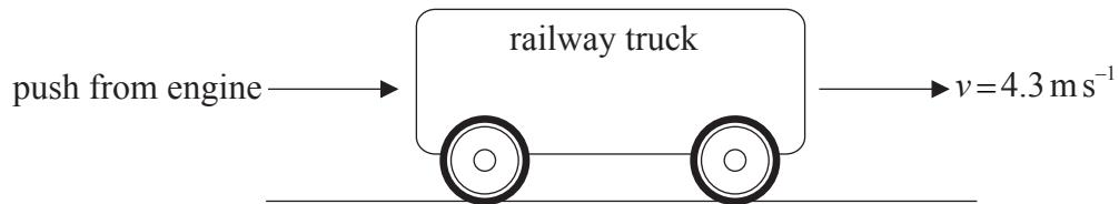
The engine is in contact with the truck for a time  $T = 0.54\text{ s}$  and the initial speed of the truck after the push is  $4.3\text{ m s}^{-1}$ . The mass of the truck is  $2.2 \times 10^3\text{ kg}$ .
