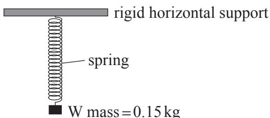
An object W of mass 0.15 kg is suspended from the other end of the spring. The extension  $x$  of the spring is proportional to the force  $F$  causing the extension. The force per unit extension of the spring  $k$  is  $18 \text{ N m}^{-1}$ .
