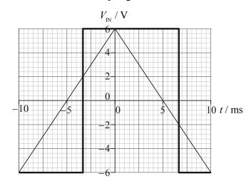
(c) digital signals are <u>distorted</u> (by noise/dispersion) during transmissions; the Schmitt trigger <u>reshapes</u> the signals;
