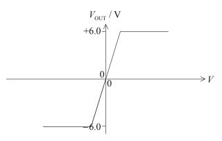
(ii) the output voltage changes abruptly from a low to a high value; depending on whether the input voltage is smaller/larger than some reference voltage;
