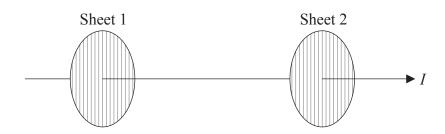
The incoming light on sheet 1 is unpolarized. The intensity of the light transmitted is I. To reduce the intensity to  $\frac{I}{2}$ , which sheet must be rotated and through what angle?
