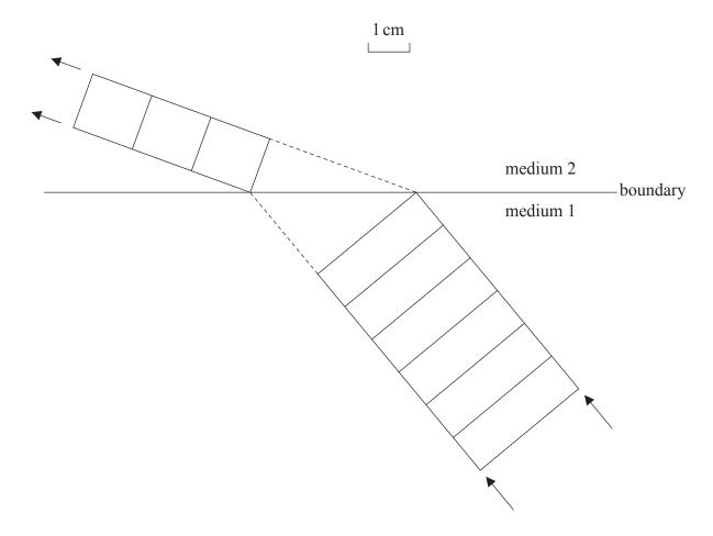
The ratio of the refractive index of medium 2 to that of medium 1 is
