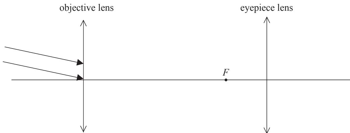
The lenses are positioned so that their focal points are at the same location, labelled *F* on the diagram.
