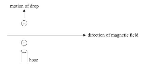
As each drop leaves the hose it becomes negatively charged. Which of the following describes the direction of the magnetic force acting on the drops?
