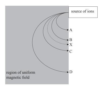
Track X shows the path of a singly-charged carbon-12 ion in the chamber.
