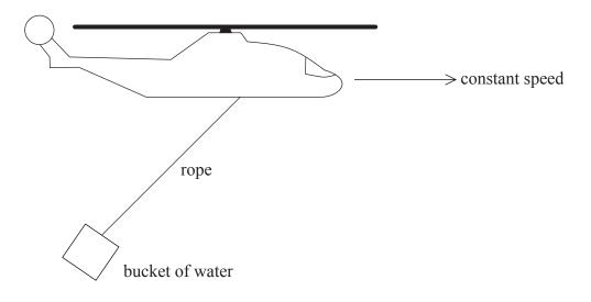
Which of the following diagrams is the correct free body diagram of the forces acting on the bucket?
