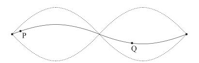
The solid line shows a photograph of the string at a particular instant of time. Two points on the string have been marked P and Q.
