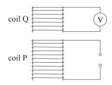
Coil Q is connected to a sensitive voltmeter. The current *I* in coil P is varied as shown below.
