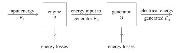
What is the efficiency of this electrical energy generating system?
